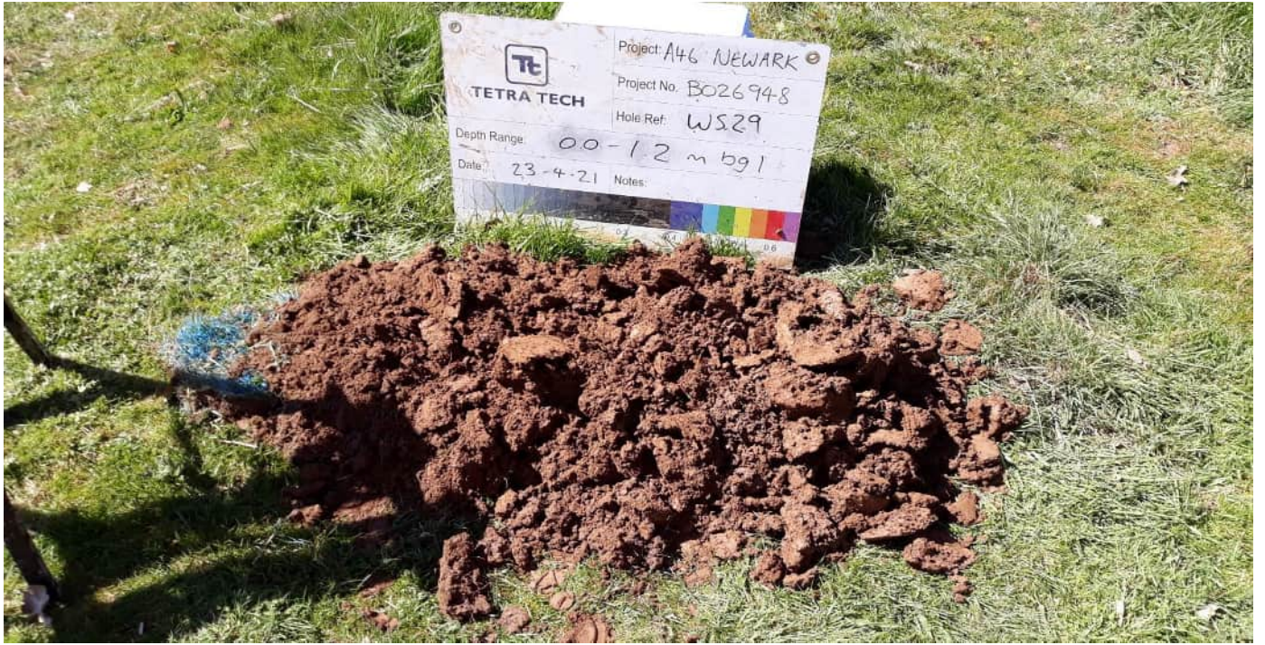
Plate 51 WS29 - Hand Pit GL to 1.20m bgl
